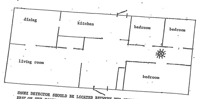
SMOKE DETECTOR SHOULD BE LOCATED BETWEEN THE SLEEPING AREA AND THE REST OF THE FAMILY UNIT.
