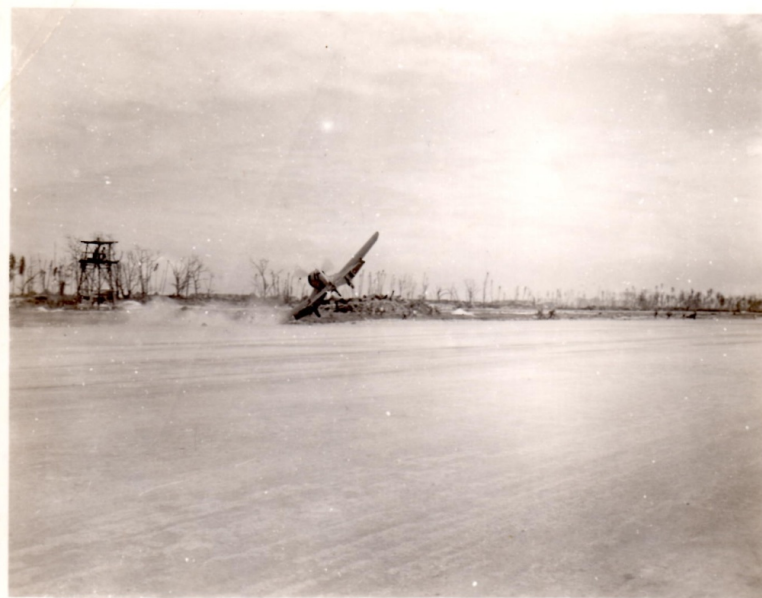
KWAJALEIN 29 FEBRUARY 1944 CORSAIR PILOT MISJUDGED STRIP AND TRIED TO PULL UP. LACKING FLYING SPEED, THE PLANE'S WING DROPPED AND STRUCK RUNWAY.
